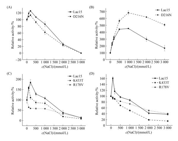
Figure 5 Dependence of the enzyme activity on NaCl for Lac15 and mutants D216N, K433T and R178V towards ABTS (A), guaiacol (B), catecol (C) and dopamine (D).
