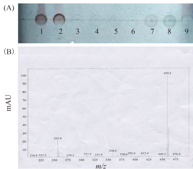
Figure 5. TLC (A) and ESI-MS (B) analysis of the hydrolysis products of colloidal chitin by Chi92. Lanes in A: 1–6, GlcNAc 6 to GlcNAc standards, respectively; 7, hydrolysis products of colloidal chitin by Chi92; 8, control; 9, mixture of GlcNAc 6 to GlcNAc standards.
